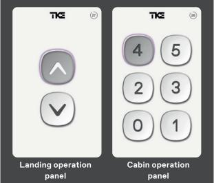
The interface is very simple and intuitive. The user only has to focus the device's camera on the QR code sticker and use the virtual keypad to generate the call to their destination floor. QR codes are unique to each installation, floor and COP. The system works on both iOS and Android devices. There is no need to download an app. To operate, internet connectivity is needed.
